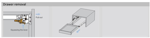
To remove the drawer, grasp the drawer on each side, squeezing the levers and pulling out and up on drawer
