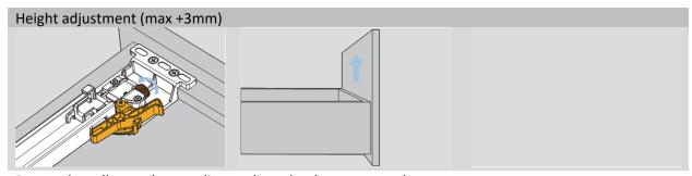
Rotate the roller on drawer clip to adjust the drawer up or down
