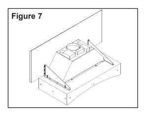
**Step 8:** Make all ventilation and electrical connections at this time. These must be done in accordance to all applicable building codes and requirements in your area.
