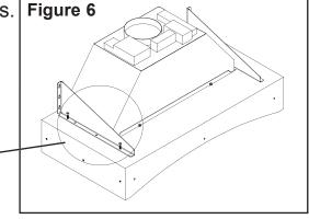
Step 7: Using help if necessary, lift the liner, Blower and mounting bracket assembly into position and hang on the screws extending from the mounting plate. Make sure the brackets are firmly seated into the key hole slot and then tighten all the screws (See figure 7).
