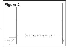
Step 3: Screw the mounting plate to the wall matching the bottom of the mounting board to the line on the wall. Make sure to hit at least two studs and to use at least 6 screws of sufficient size and length for the application (See figure 3).
