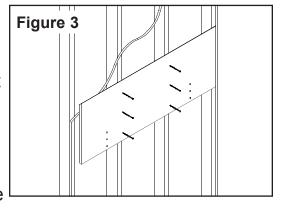
**Warning**: Failure to fasten this panel to studs or using the wrong screws may cause a failure of the mounting system and possible injury.
